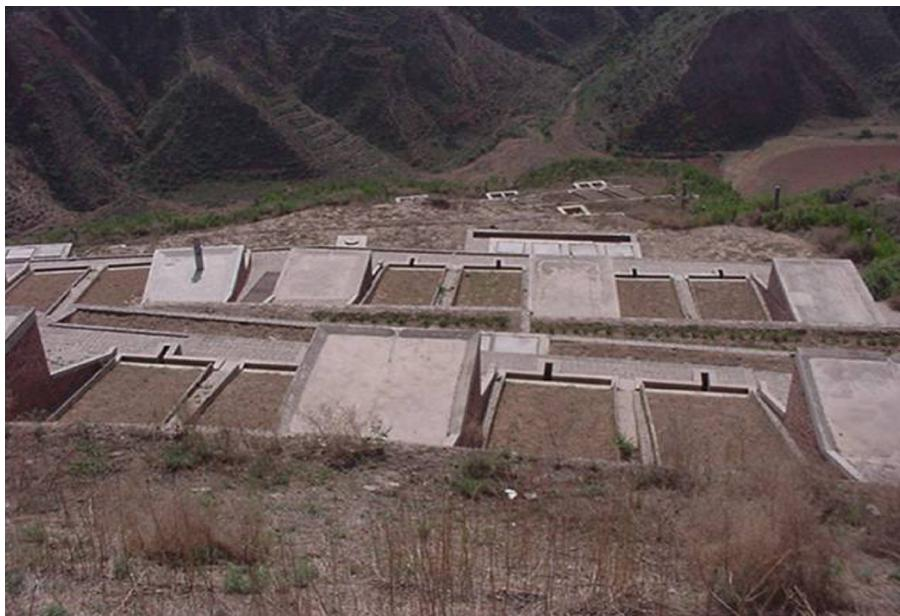
**Fig. 3.** Short slope plots (SSP) with a dimension of 2 m wide and 7 m long at slope angles of  $5^\circ$ ,  $10^\circ$ ,  $15^\circ$ ,  $20^\circ$ ,  $25^\circ$ , and  $30^\circ$ .
